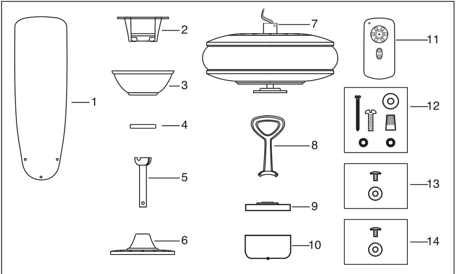
1. Fan blades (5) (Model: TB60-xx, packed in separate box.) (CAUTION: This GLADIATOR (GL3) Ceiling Fan must only be used with the Models "TB60-xx, W154, W354 and 56" Décor Match™ Blades, it is not intended to be used with any other REGENCY® Fan blades.)
